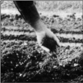
The standard field test for binding characteristics of gravel with moisture is squeezing a handful into a ball.
