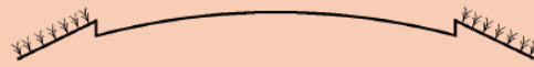
Roadway with parabolic crown. The outer edge of the road slopes too much. Gouging causes high shoulder, and center 1/3 of the road tends to be flat.
